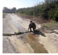
Figure 2: KVA storm water run-off sampling
