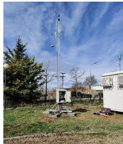
**Figure 13: Noise monitoring terminal at Thessaloniki (SKG) airport (MP01)**
