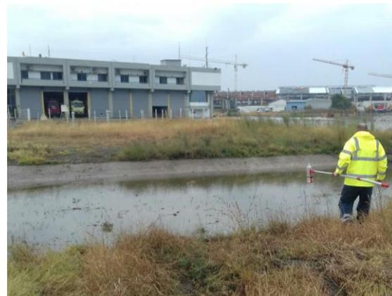
Figure 9: SKG storm water runoffs sampling, with the use of a bailer
