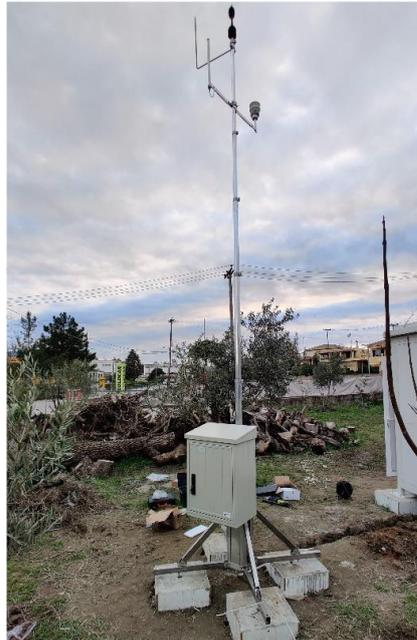
**Figure 9: Noise monitoring terminal at Corfu (CFU) airport (MP01)**
